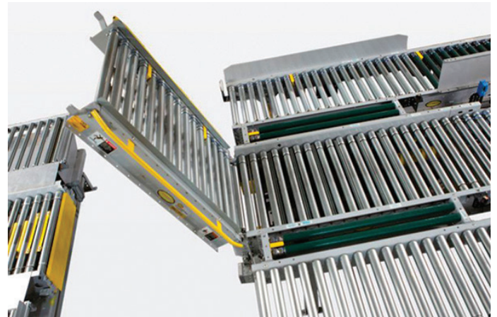
Gates are available for use with a variety of conveyors. Gates provide a passageway for personnel, lift trucks, and other equipment. Manual and gas power gates are available.
